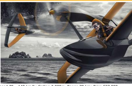
Wingspan 5m; Max T/O wt 200 Kg; Speed 70 - 140 km/h; Ceiling 3,000m. Range 70 km; Price €27,000
